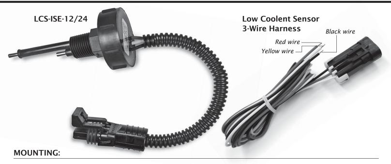
The sensor can be mounted in surge tanks as well as heat exchangers and radiators, utilizing a high temperature PPS or Polyphenoline sulfide thermoplastic with a 3/8-inch pipe thread. Surface mount technology and circuit filtering have made the sensor compatible with current vehicle demands for performance guided by SAE standards. The sensor operates on both 12 and 24 VDC electrical systems.
